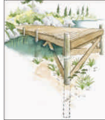
Figure 8: Permanent Post Dock
