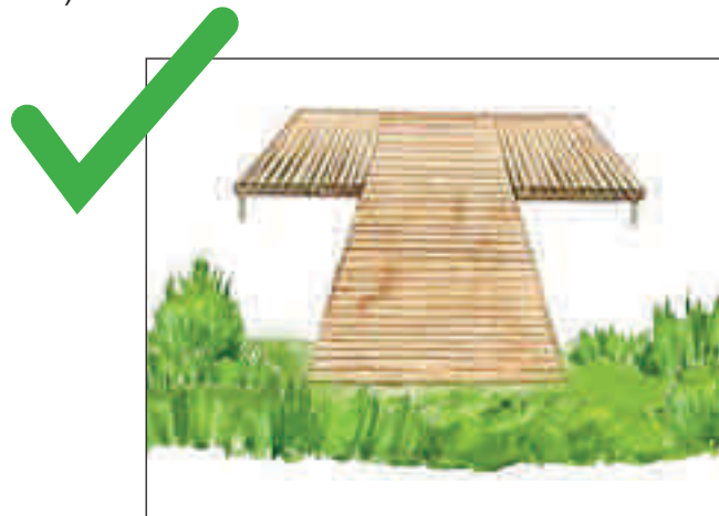
Figure 3: Dock oriented away from shore
