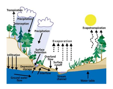
The water balance for the watershed (or subwatershed) determines the amount of water available for water ecosystem functioning and the amount available for human uses.
