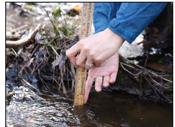
CSW volunteer measuring hydraulic head, a measurement of surface flow velocity
