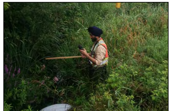
RVCA staff member using a YSI probe to measure the water chemistry of a headwater drainage feature during a summer site visit
