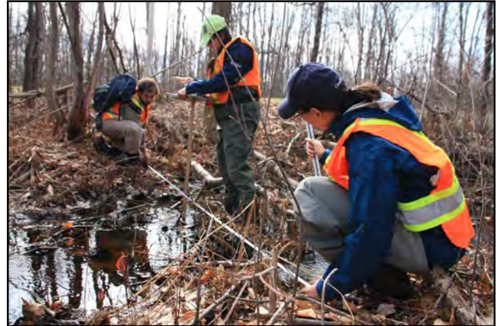
Volunteers measuring the wetted width of a headwater drainage feature
