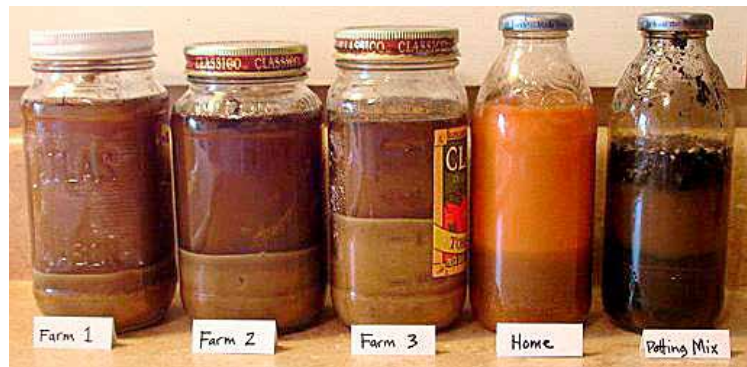
Figure 6: Measuring soil after it settles in a jar.
